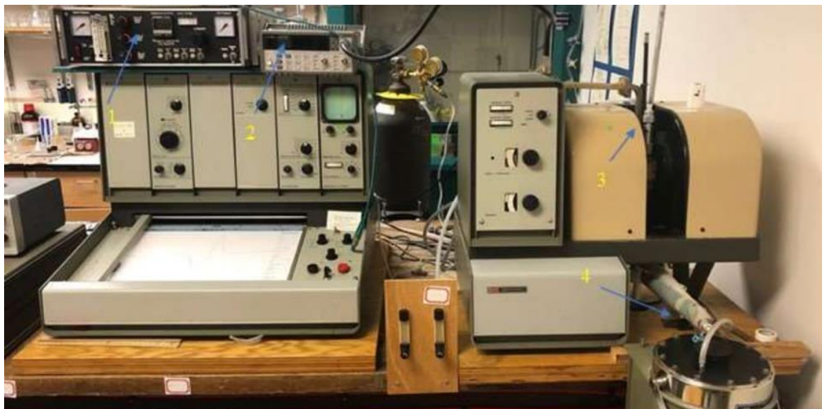
Figure 3. Instrument Setup Varian E-3 X-band Spectrometer. D.Petasis Lab, Allegheny College. 1- Temperature controller, allows us to monitor the temperature and control Nitrogen flow during low temperature run. 2- Universal counter: displays the frequency, \nu , throughout the run. 3- Cavity: where samples are placed. 4- Dewar: stores liquid nitrogen that is supplied to the cavity for cooling it down during low temperature EPR runs. (D. T. Petasis and M. P. Hendrich, 2015)
